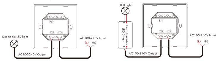
Note: When calculating the maximum number of load lamps or drivers, the input power or input current parameters of a single lamp or driver must be used, the output power parameters can not be used.
